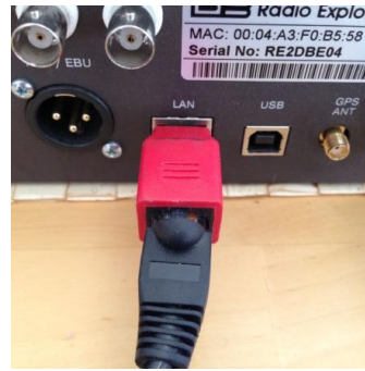
Ethernet crossover adapter in place
