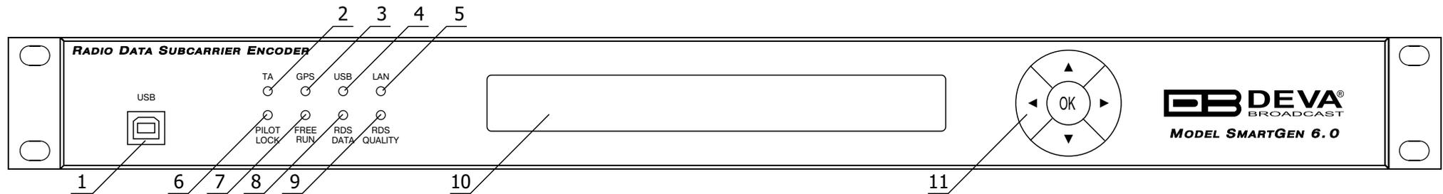
1. **USB Connector** - B-Type, for interconnection with PC / USB 2.0 Communication Port
