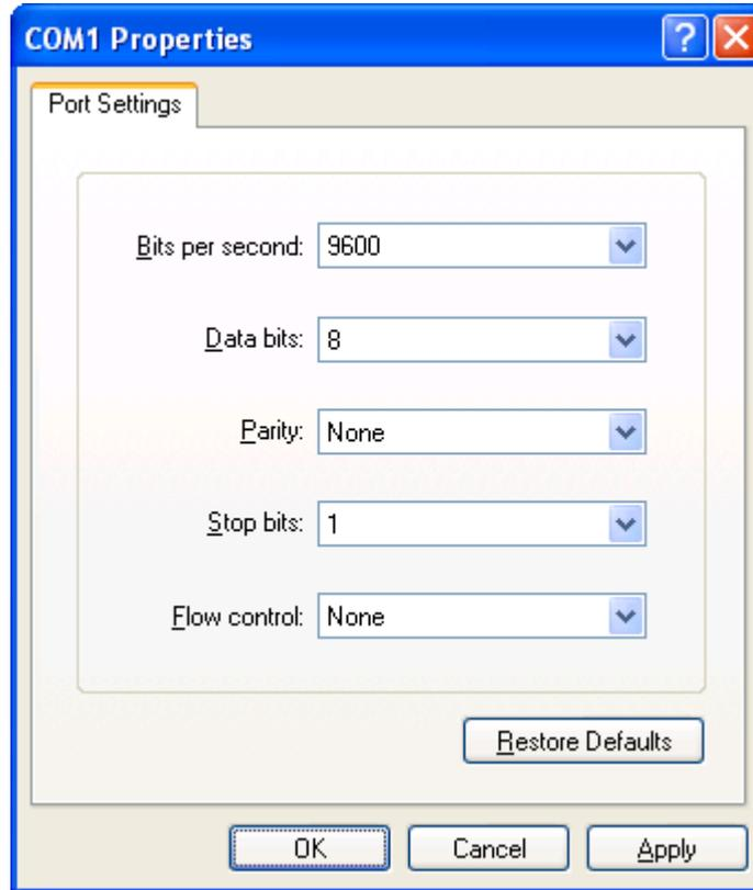
If you experience trouble communicating with the SmartGen 6.0, there's a quick and easy check to verify that the computer and the terminal program are functioning normally. With pins 2 and 3 of the DB-9 connector shorted with a screwdriver, whatever is typed on the keyboard should appear on the screen.
