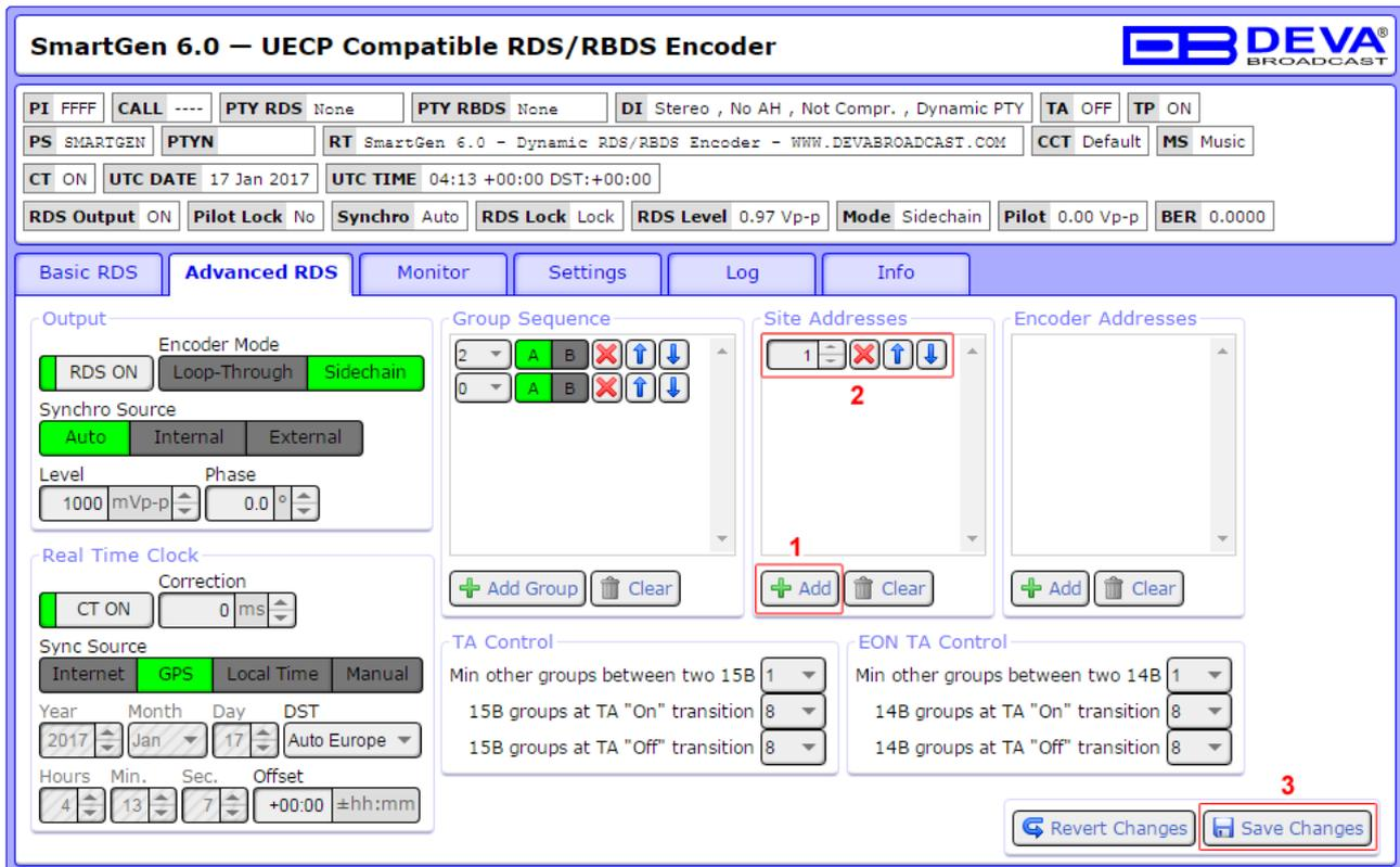
The screenshot shows the 'Advanced RDS' configuration page. The 'Site Addresses' section contains a list with two entries: '1' and '2'. Red boxes highlight the '+ Add' button at the bottom of the list, the '2' entry, and the 'Save Changes' button at the bottom right. Red numbers 1, 2, and 3 are placed next to these elements respectively.
