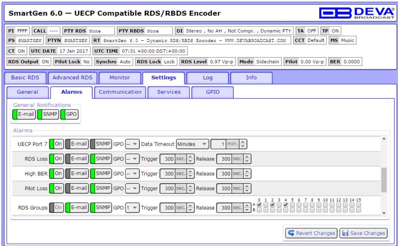
**General Notification** – Generally enables the type of notification/s to be used in case an alarm event is generated.
