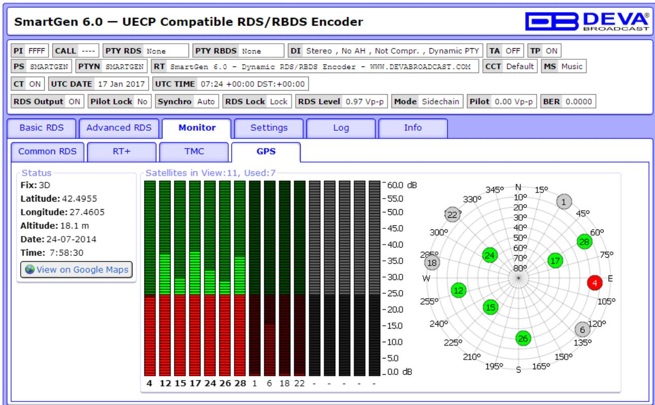
GPS should be chosen as “Sync Source” in order for the GPS to be available. The “Sync Source” is set in the “Advanced RDS” tab ([see “Advanced RDS” on page 64](#)).
