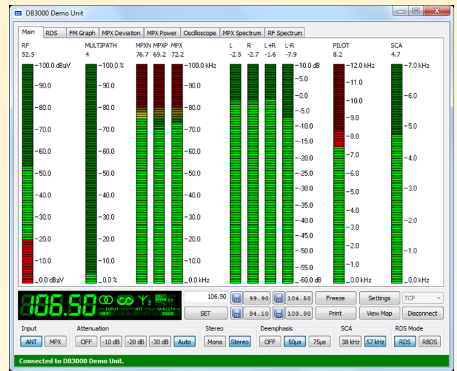
Main Device View with all mandatory parameters as LED readings
