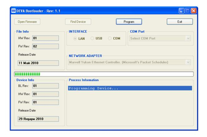
10. Firmware Upgrade completion is indicated by the progress indicator and in *Process Information* area as shown on the picture below:
