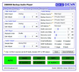
DB8008 has one main and three backup audio sources. If the audio signal of the main source disappears the device will switch to the first available backup source.
