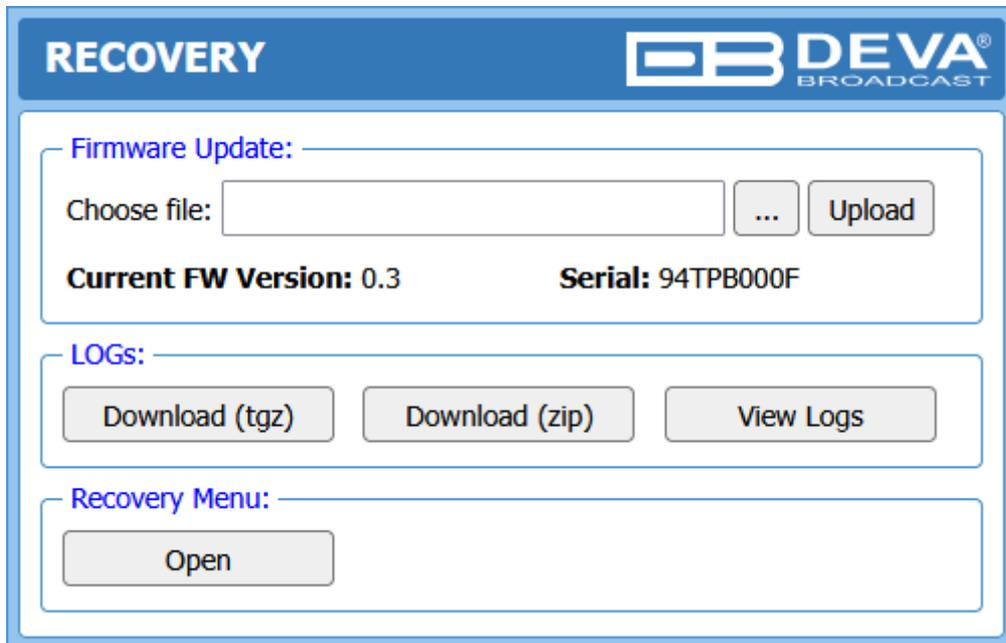
The screenshot shows the 'RECOVERY' interface with the DEVA BROADCAST logo. It features three main sections: 'Firmware Update' with a file selection field and an 'Upload' button; 'LOGs' with buttons for 'Download (tgz)', 'Download (zip)', and 'View Logs'; and 'Recovery Menu' with an 'Open' button. The current firmware version is 0.3 and the serial number is 94TPB000F.
