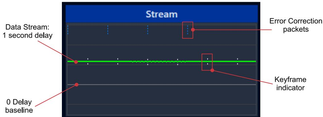
The Stream Display provides a visual health indication of the incoming MicroMPX data stream. Adjustments made in the Encoder's **Error Correction** settings directly influence this display. The Stream Display contains the following visual indicators:
