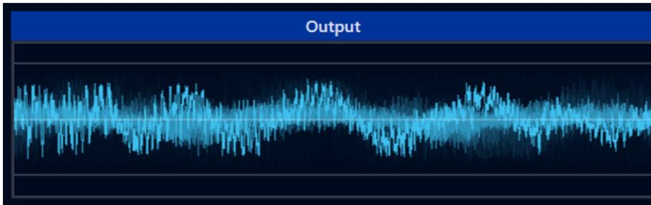
The Waveform Display provides a real-time visual representation of the program signal.
