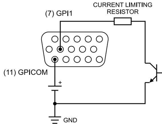
Figure 1-1 - External Power Supply
