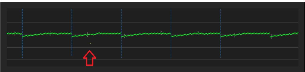
If you see occurrences like this, you can see that the yellow packet was recovered only just in time, and that could be a reason to increase the Delay a bit. Or reduce the forward error correction span setting.
