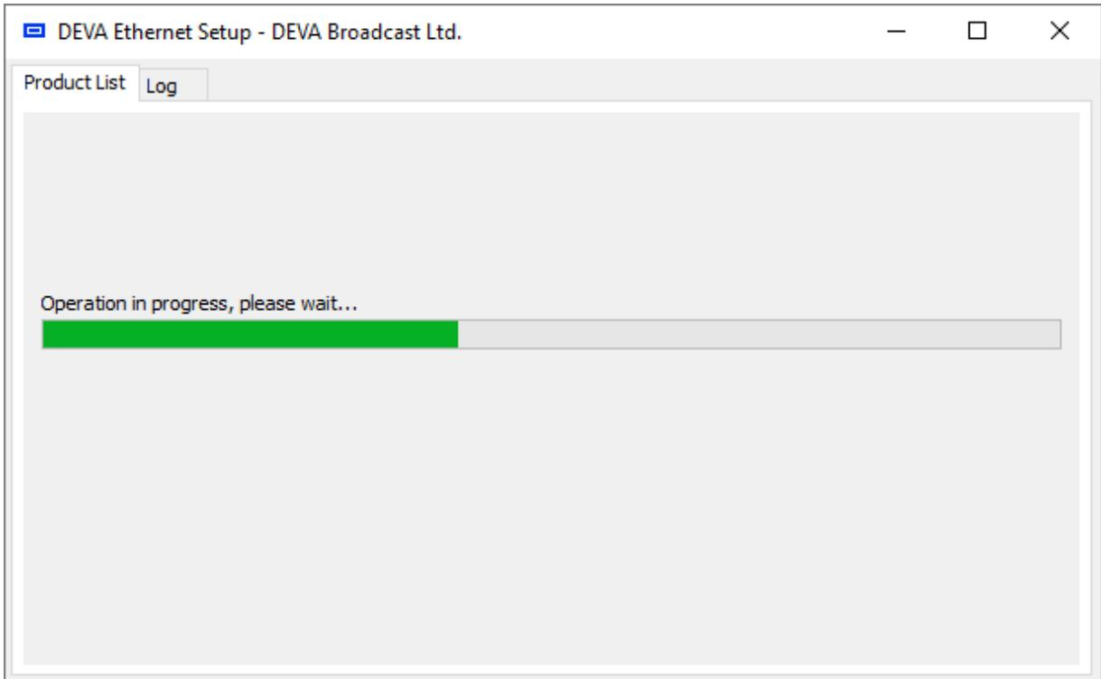
5. A new network scan process will be performed automatically to confirm that the applied settings are accepted.
