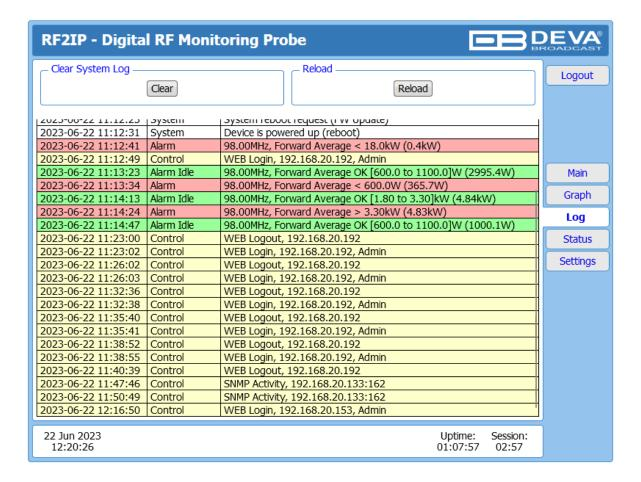
Here are listed all the Device System Events. The local measurements and logs are saved in RF2IP's volatile memory and are automatically deleted upon power loss.
