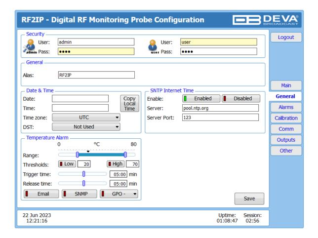
RF2IP provides you with protected access to the device settings. You can choose between two types of log in.
