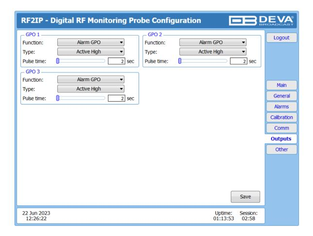
This section of the WEB Interface, allows you to set Function, Type and Pulse time for each GPO.
