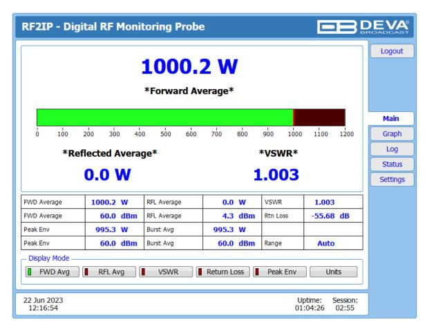
The RF2IP has two inputs and measures both the forward and the reflected power.
