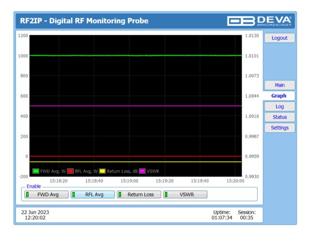
The Graphs page represents the value deviation of measured parameters in time. All the parameters are color coded and can be enabled or disabled depending on the preferences.
