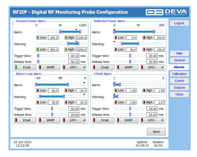
RF2IP has a set of the 4 parameters that can be monitored: Forward Power, Reflected Power, Return Loss and VSWR. Trigger and alarm release times can be set for each alarm. The notification means (Email, SNMP and GPO) is set for each parameter individually. To enable the notification, press on the relevant button so that it could be illuminated in green.
