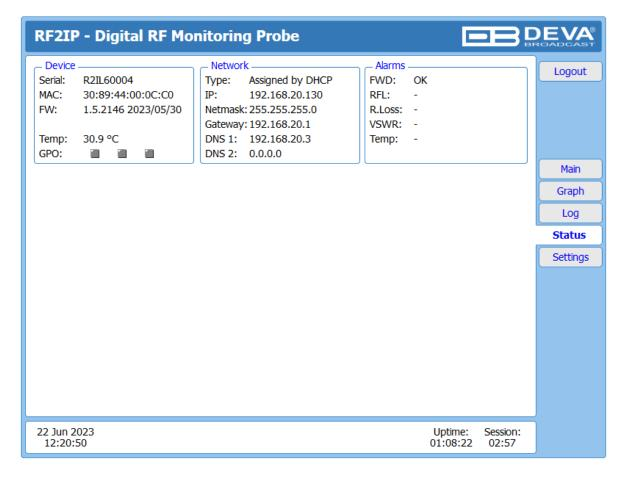
The status tab shows the alarm status of the RF2IP, along with the basic device and network status (IP address, MAC, etc.).
