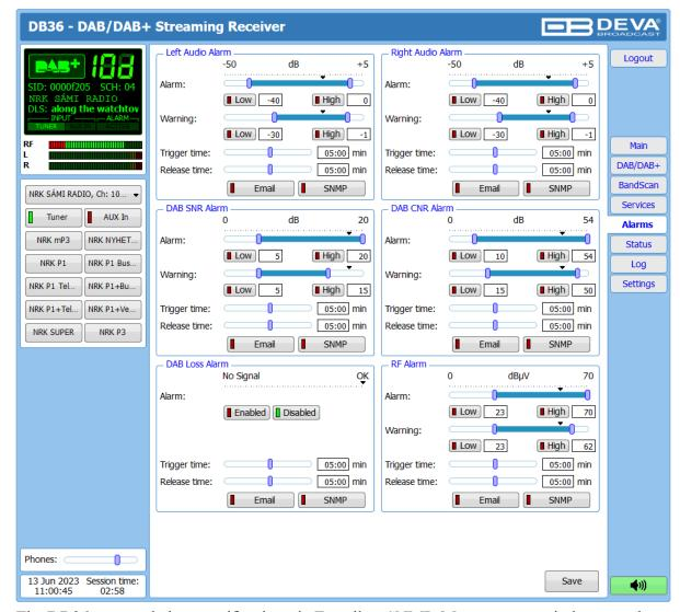
The DB36 can send alarm notification via E-mail or SNMP. Measurement windows can be set for each of the six parameters: RF, Left and Right audio levels, DAB Loss, DAB SNR, DAB CNR. Trigger and alarm release times can be set for each alarm.
