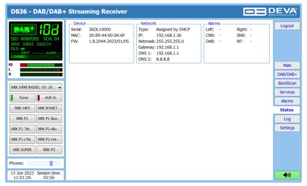
The status tab shows the basic Device, Alarm and Network statuses (IP address, MAC, etc.).
