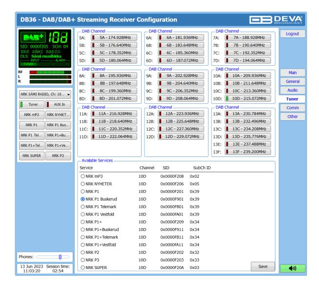
The Tuner Section gives control over Tuner settings, allowing you to select a DAB channel and service. All available services will be listed below once the list is collected from the multiplex data.
