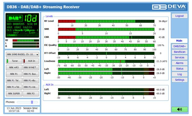
The main screen contains information on the mandatory parameters for the currently selected DAB/DAB+ station, represented as LED readings.
