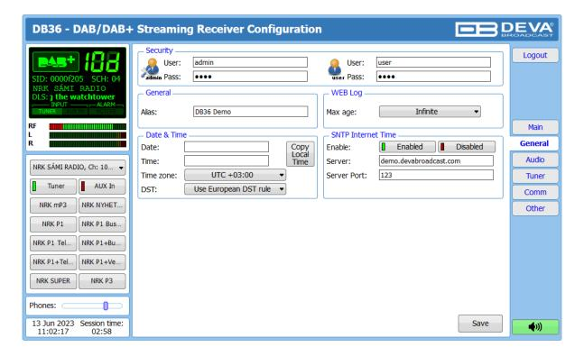
DB36 provides you with protected access to the device settings. You can choose between two types of log in.
