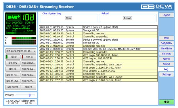
Here are listed all the Device System Events. The local measurements and logs are saved in the internal device memory. All log files can be downloaded via the built-in FTP server. For information on how the connection between the DB36 and an FTP Client should be configured, please refer to "Download files via FTP" on page 38.
