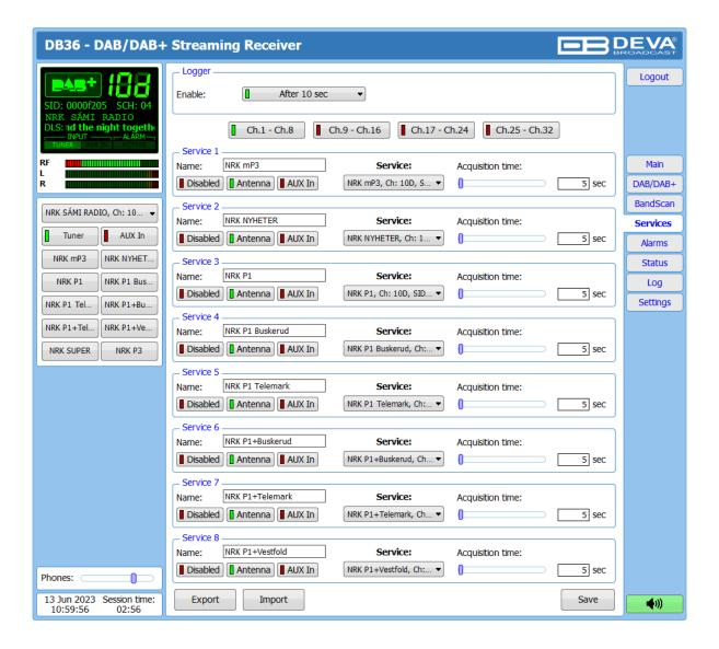
This section of the WEB Interface allows up to 32 services to be chosen and monitored, by applying the needed settings.
