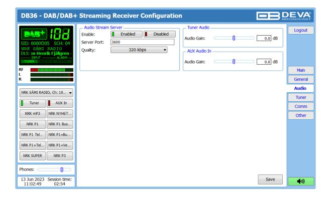
The Audio section of the WEB Interface allows the user to apply the needed settings to the Audio Stream Server, Tuner Audio and AUX Audio In of the DB36.
