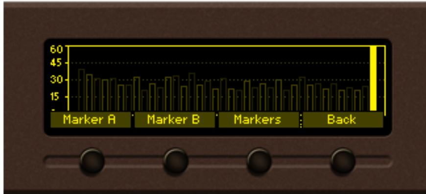
**For example:** When the following menu is selected pressing *SB3* will change the screen from Marker to Span control and vice-versa. All Soft button labels will change according to the sub-menu. The control state of the page will change upon every *SB3* pressing. Pressing the *OK* button either in Marker or Span control state will make the transition to Parameter control state. The screen will be visible until the *OK* button is pressed again or the timeout of 2 seconds elapses.
