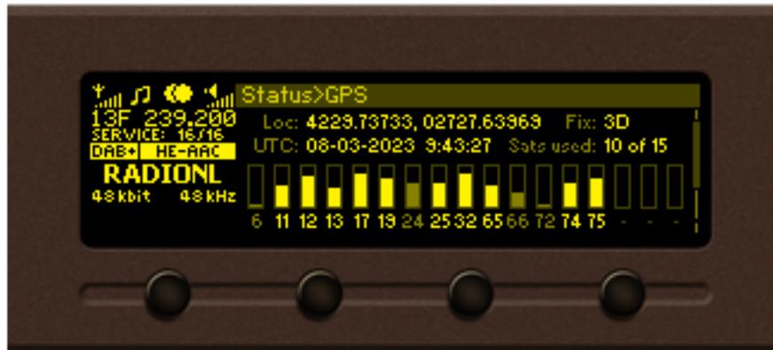
**Loc:** The current location of the device - Longitude and Latitude in degrees.
