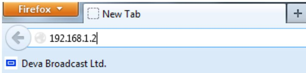
**NOTE:** Due to the inability of some WEB Browsers to read the IP address format displayed on the screen of the device, the numbers included in the IP Address must be written without the leading zeros. For example: 192.168.020.095 must be written as 192.168.20.95
