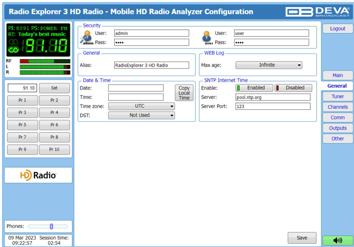
Radio Explorer III HD Radio provides you with protected access to the device settings. You can choose between two types of log in.
