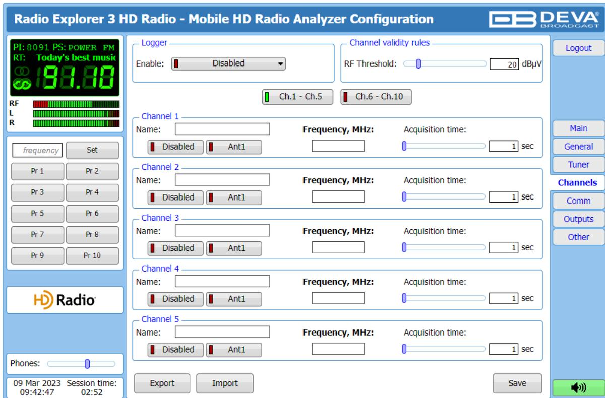
Trough this section of the WEB Interface, up to 10 radio frequencies could be chosen and monitored, by applying the needed settings. When the desired adjustments are made, Radio Explorer III HD Radio will monitor all of the selected frequencies at regular intervals. All of the collected information is accessible through the built-in FTP Server;
