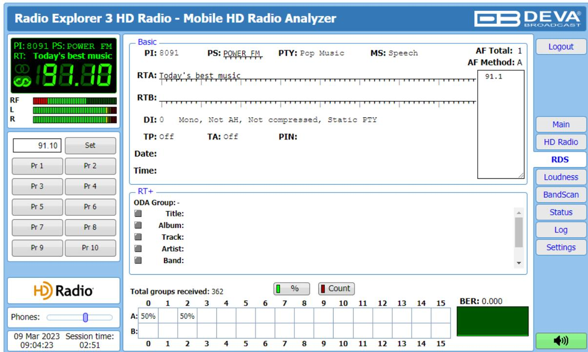
All basic elements of the RDS/RBDS are displayed on the screen – PI, PS, RT, TA/TP, etc. Represented a list, also available are the Alternative frequencies (AF). Radio Explorer III HD Radio supports one of the most used ODA Applications - RT+ (Radio Text Plus). If your radio station has RT+, Radio Explorer III HD Radio will display the information.
