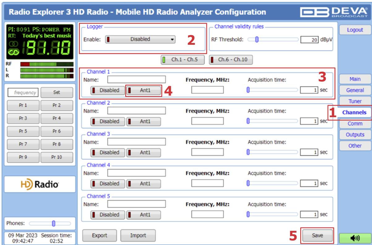
1. Open the main application window and go to **Settings> Channels** tab;
