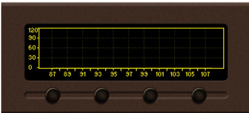
To ensure better reading of the data plot, the Header area and the Soft Buttons labels will be hidden automatically a short time after the soft button is released. Pressing a button will display the function labels again.
