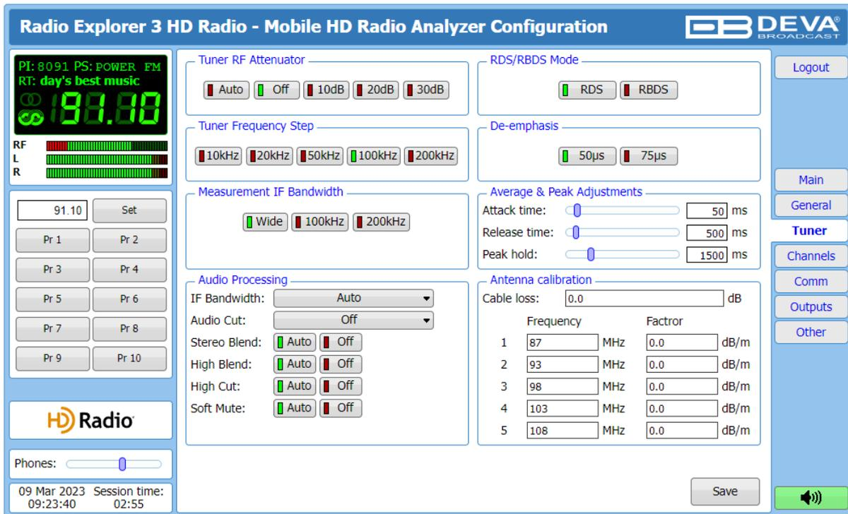
The Tuner Section gives full control over the RF Antenna Input, Tuner and Audio Processing settings.
