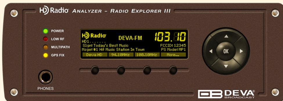
The Radio Explorer III HD Radio measures all important signal parameters, including the RF level, MPX deviation, Left & Right Audio levels values, as well as HD Radio® parameters such as DAAI and CDNR. Additionally, it boasts a Loudness meter, which can be shown as defined by ITU BS.1770-4 and EBU R128 recommendations, as the product supports both.
