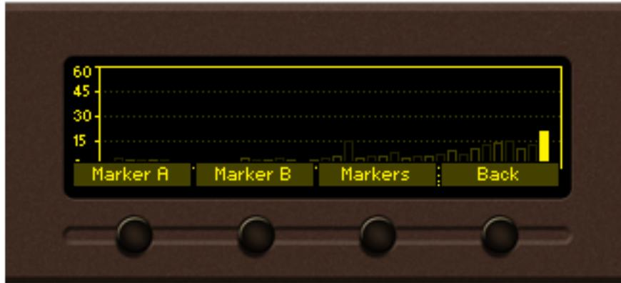
For example: When the following menu is selected pressing [SB3] will change the screen from *Marker* to *Span* control and vice-versa. All Soft buttons labels will change according to the sub-menu. The control state of the page will change upon every [SB3] pressing.
