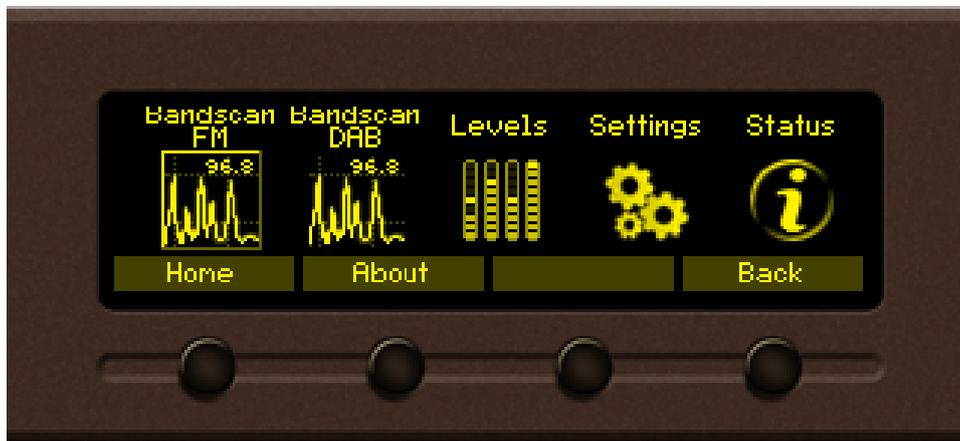
Press the [OK] Button to enter the “*Status*” section. Via the Front panel navigational menu press the [DOWN] button.
