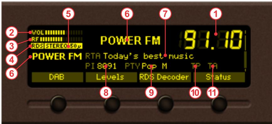
1. Frequency Indicator, showing the currently selected frequency, in MHz;
