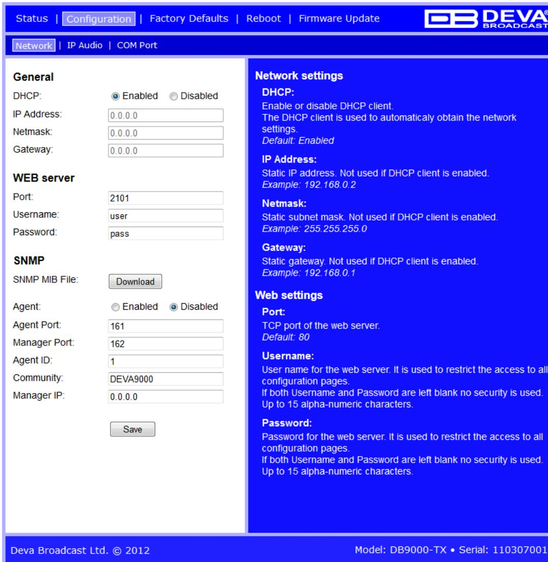
The screenshot shows the configuration page for the DEVA DB9000-TX device. The interface is divided into several sections:
