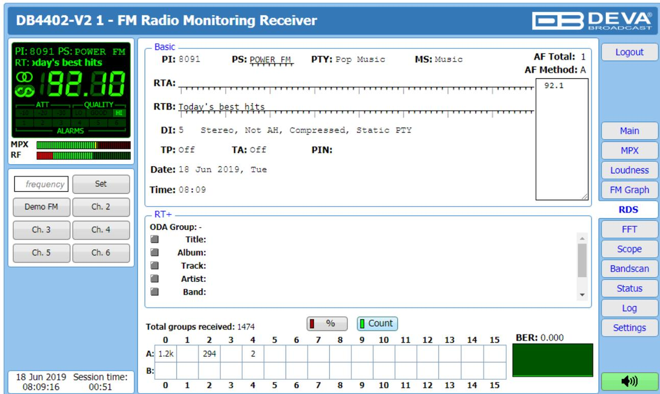
The screenshot shows the RDS/RBDS monitoring interface for the DB4402-V2 1 FM Radio Monitoring Receiver. The interface is divided into several sections:
