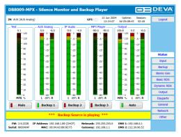
The Status screen contains information about the source levels. You can easily select the preferred audio source by using the source selection buttons. By selecting the interactive [Auto] button, the DB8009 will automatically select audio source in accordance with the applied Audio Backup Settings.
