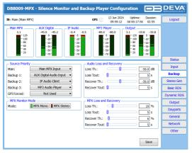
The backup sources priority is user-defined and can be set through the Source Priority section. If the audio from the main source disappears, the DB8009 will automatically switch to the first backup source; if it also fails, the unit will switch to the second. Once a source with higher priority is restored, the unit will switch back to it.
