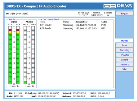
Upon opening the WEB interface, the main Status window will appear. The page contains information on the device's current status - the LED bar-graph representation of the left and right Digital and Analog audio levels in dBFS, as well as the Active connections - Type, Status, Remote Peer and Codec.
