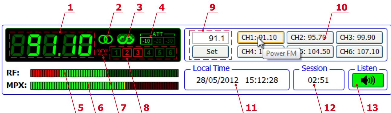
1. Frequency indicator showing currently tuned frequency;
