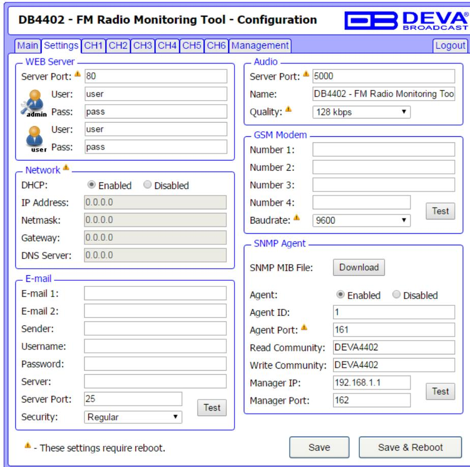
**DB4402 - FM Radio Monitoring Tool - Configuration**
