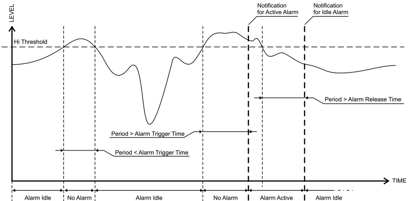
If RDS Group has not been received for more than Alarm/Warning Trigger Time state is changed to Active. If state is Active and Release Time has elapsed and the RDS Group is received state is changed to Idle. If the RDS Group is received before the Release Time is elapsed state remains Active.
