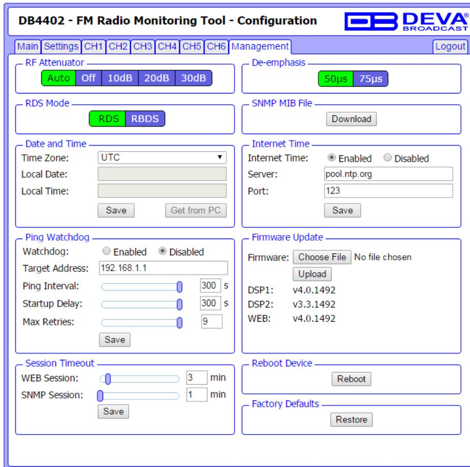
The screenshot displays the 'Management' configuration page for the DB4402 FM Radio Monitoring Tool. The page is organized into several sections:
