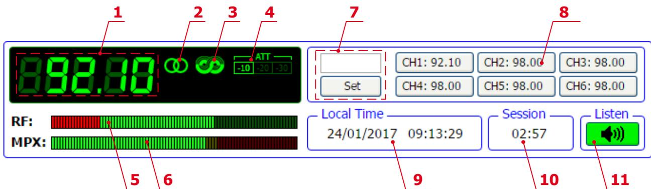
1. Frequency indicator showing currently tuned frequency;
