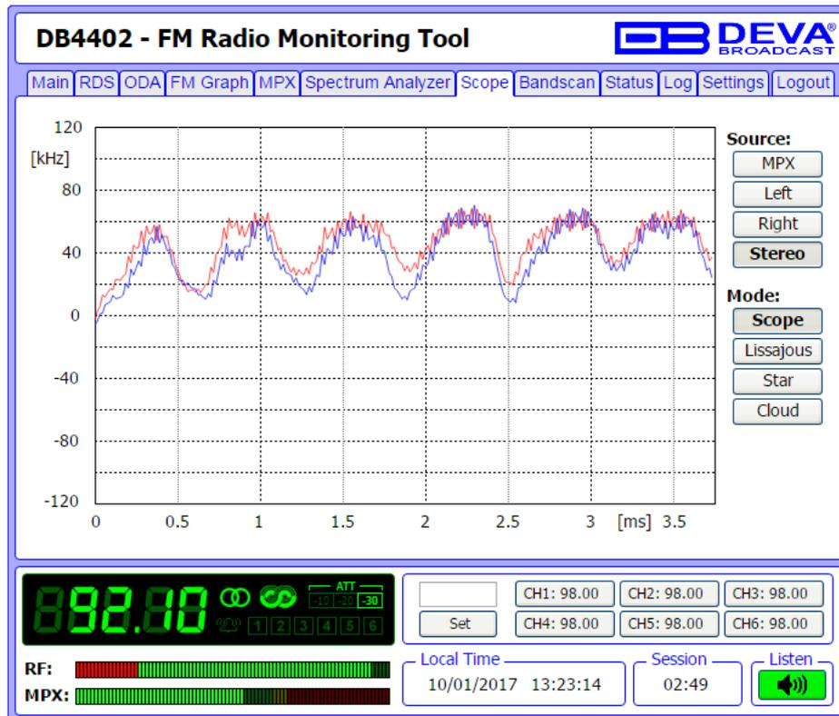
SCOPE screen represents the signals participating in the process of demodulating and stereo decoding over time. In order for the signal source to be changed, the corresponding button on the right-side of the graph should be pressed.
