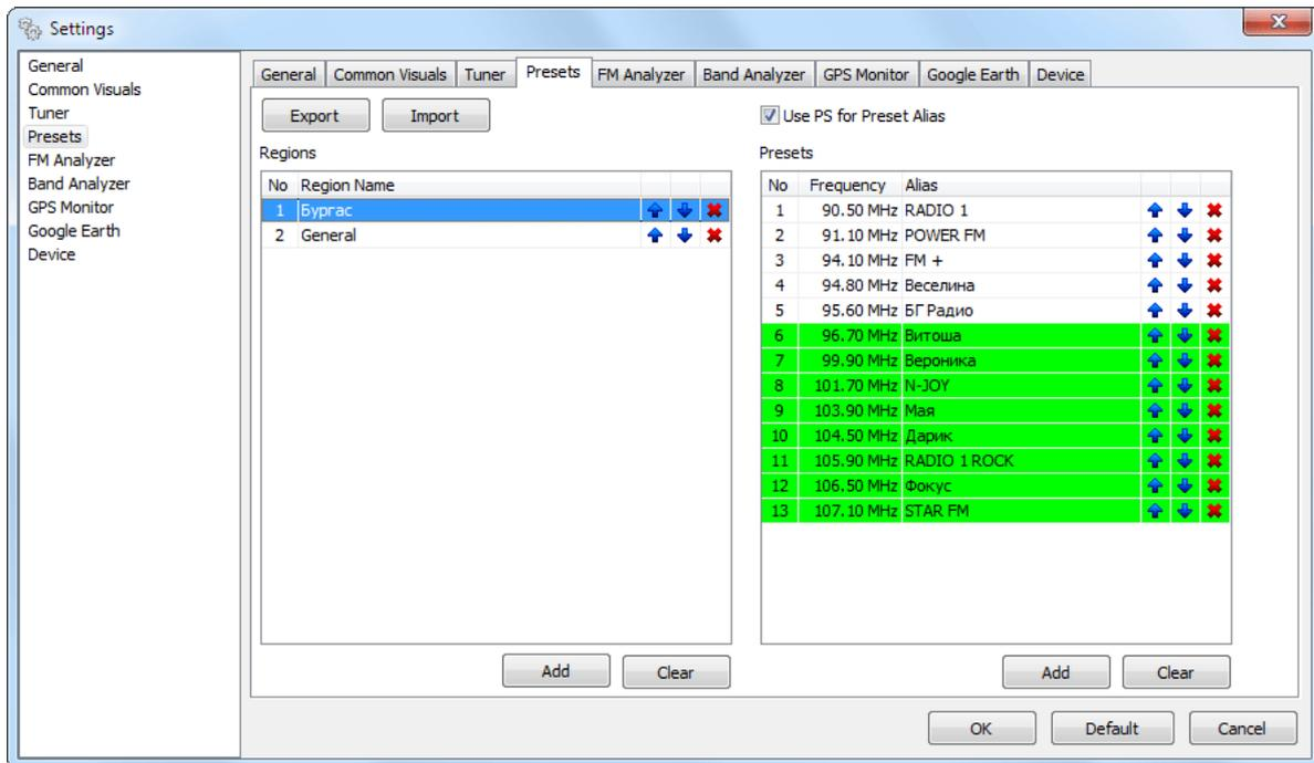
Using this feature you can assign easy to access memory presets (see “FM Tuner, Modes and Presets” on page 43)[15,16,17,18]. Frequencies assigned here, correspond directly to the quick preset buttons situated along with the rest of the tuner controls. Intended to serve as a quick access to favorite stations, preset button needs no more than a click. Presets can be assigned from here as well as from Quick Save buttons. Saving and Recalling is very easy which explains why they are “Quick Presets”.
