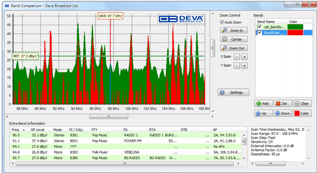
The main purpose of this tool is to provide easy way for visual comparison between different spectrum plots. The tool utilizes BND files, which are saved previously from Band Analyzer ([see “Band Analyzer Results Saving” on page 52](#)). The tool overlays different spectrums but is indifferent about comparison itself, which is granted entirely to user.
