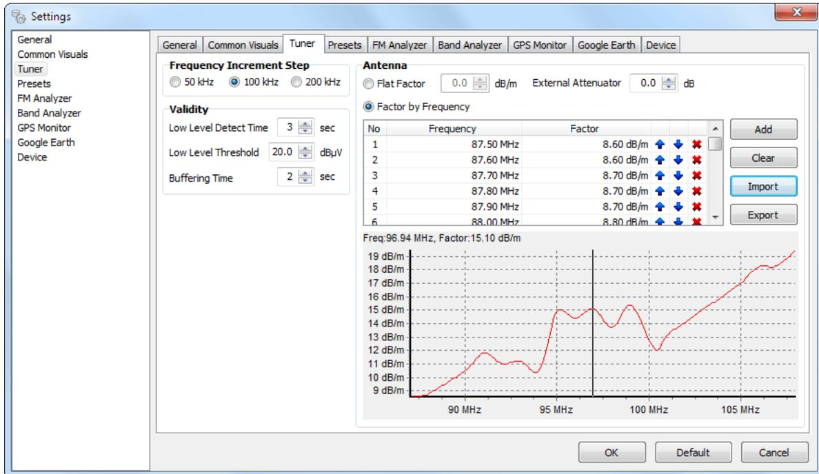
**Frequency Increment Step** – You can choose the frequency adjustment step. Usually it is 100kHz for Europe and 200kHz for the US
