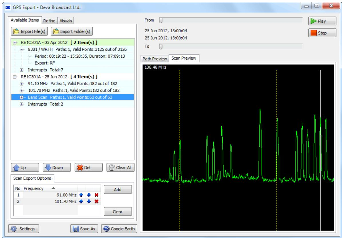
Additionally the Frequency Campaign could give one Cyclic Band Scan, which is made at the end of every Frequency List Cycle.
