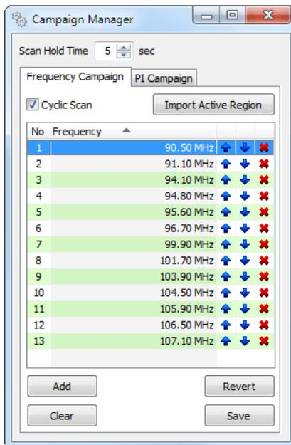
Frequency Campaigns has no special rules. Their purpose is to observe station parameters and switch to next station in list. Suitable for small region surveys, which presumably did not require regional station switching.
