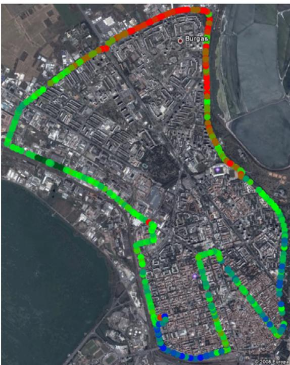
While examining points, Data Coloring takes its place. As individual every Point is Color-Coded according to Value measured and gives fast perception about parameter's condition. As group of Points Color-Coding represents per-area affect of the parameter.
