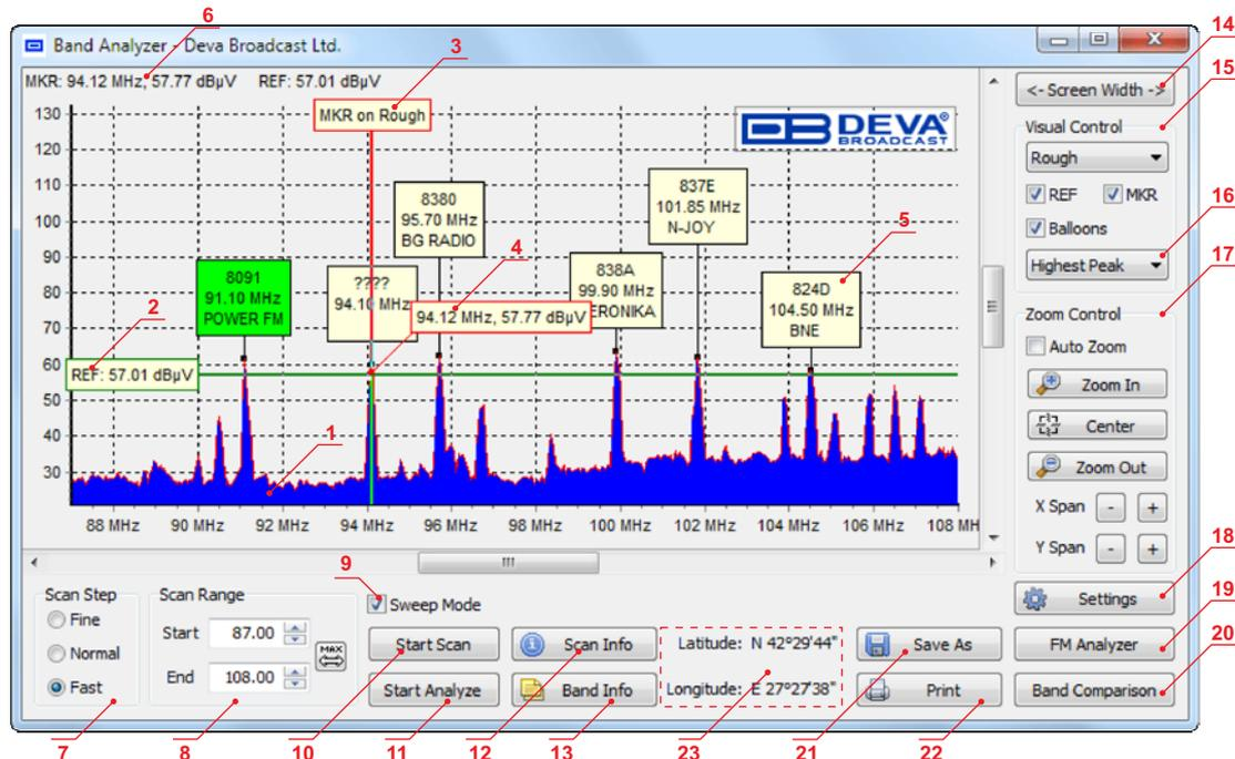
**1. FM Band Spectrum.** The horizontal scale shows the frequencies. The vertical their measured levels.
